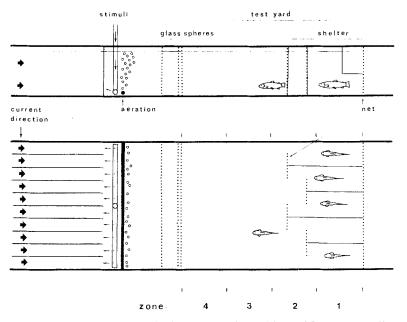
FIG. 1. The modified test area of the fluviarium. The positions of fish were usually noted as shown in the figure except when there was a supply of stimuli inducing the charr to swim upstream. The dominant individual was commonly located in front of screens which functioned as shelters to subordinate fish. Four zones used for analyzing upstream movement of fish were defined by lines on the bottom transverse to the direction of flow.
