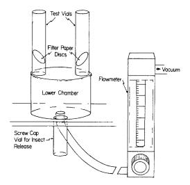
FIG. 1. Dual-choice olfactometer for the boll weevil. See text for details.
