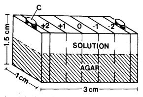
FIG. 1. Linear channel, barrier design of polycarbonate chamber used in pheromonal studies. Reprinted from Imperia et al. (1980) with permission of *The Journal of Parasitology*.
