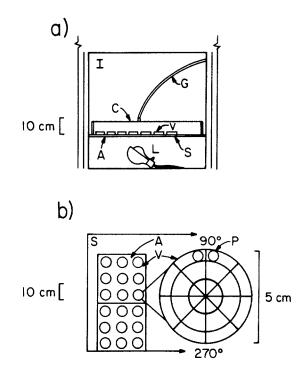
FIG. 1. Experimental apparatus for testing in vitro chemical orientation of *S. mansoni*. (a) Side view; A = acetate sheet marked with grid coordinates; C = Plexiglas cover; G = gas line; I = incubator; L = light; S = Plexiglas shelf; V = vessel; (b) top view showing enlarged view of vessel with grid coordinates; P = agar plug position. Parasites were placed in the center of the vessel.
