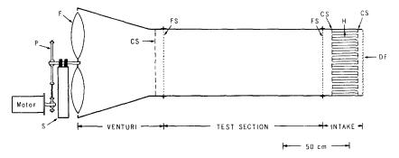
FIG. 1 Lateral section of the flight tunnel: H, honeycomb of 6-mm-diam. soda straws; CS, course screen  $(7 \times 7 \text{ mesh/cm}^2)$ ; FS, fine screen  $(13 \times 13 \text{ mesh/cm}^2)$ ; DF, dust filter; F, fan blade; and S, fan support.
