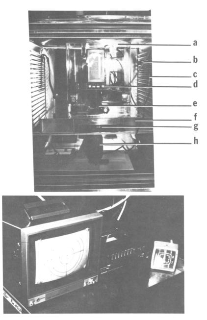
FIG. 1. System employed for time-lapse video tape recording of the responses of schistosomes to chemoattractants during cultivation in vitro. Upper photograph: (a) plastic waterproof camera housing; (b) mixed-gas line; (c) camera remote control cable; (d) camera; (e) lens system; (f) culture chamber; (g) culture vessel; and (h) light source. Lower photograph: monitor, video tape recorder, and timer.
